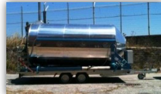
Digestore anaerobico mobile (6 m<sup>3</sup>)
